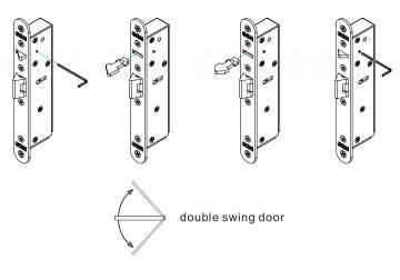
Single action door or double action door is changeable with a NIB. We provide the optional spare NIB for "**single swing door**" in case of necessary.
